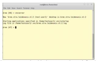
Verify that this display number corresponds with the one use have defined in the tunnel. If not, go back to 2. and add the correct tunnel. Leave the putty ssh session on.
