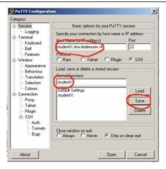
5. To use this tunnel, log into your machine with Putty. Once logged in you need to start a vncserver on the remote machine. It will respond with the display number:
