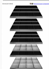
The hardware is bought for expansion. Currently the disk extension box acquired contains 20 disks, and can easily be extended with additional disks to a total of 60 disks. So the current 83TB can be extended to about 250TB by simply acquiring more disks. When the disk cabinet is filled an additional cabinet could store an additinal; 250TB of space without any major change to the hardware configuration.
