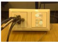
Before one can start with any displaying, the LG screen needs to be switched on. This can be done by pressing the top row 'On' button on the desktop switch board. You will see that the 'On' button is blinking for a while, until the display is fully switched on.
