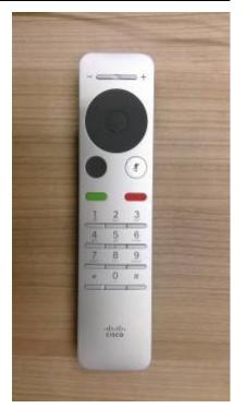
With the top part of the remote control one can step to other clickable elements in the display. Walk down to the green button to open the Call Assist window. One can select (press) a button by hitting the central Enter button in the middel of the arrow keys on the remote control.
