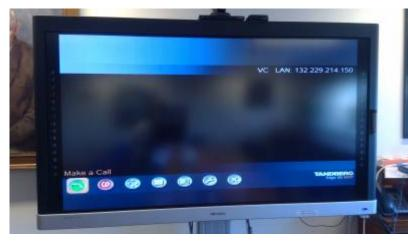
You can now type in a remote IP number to connect to another Video Conferencing unit (the . in the IP number can be replaced with a \*. After typing the IP address, you press the green pickup button on the remote to establish the connection.
